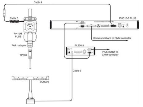
PI 200-3 with PHC10-3 PLUS interconnection with PH10M PLUS and SCR200
