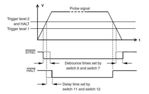
SYNC and HALT signal timing for a TP200 gauge point
