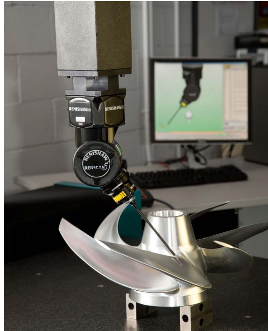
Renscan5™ allows TURBOCAM to do continuous, automated measurement of complex turbomachinery components, collecting thousands of points to verify form
