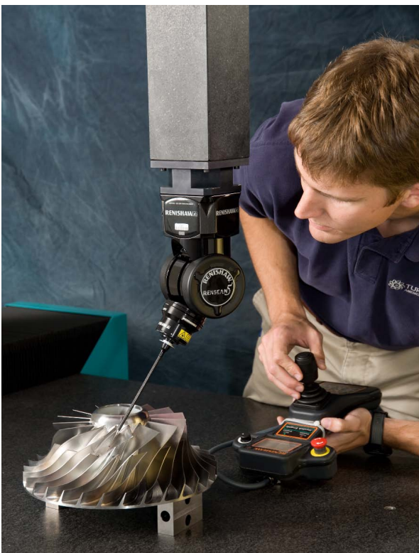
Nick Dean, TURBOCAM Product Engineer/CNC Programmer, uses teach points to create a five-axis program for inspection of a shrouded impeller
