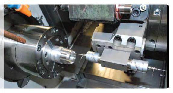
The success the company achieved using on-machine probing on its VMCs spurred it to apply probing to turn-mills such as this one.
