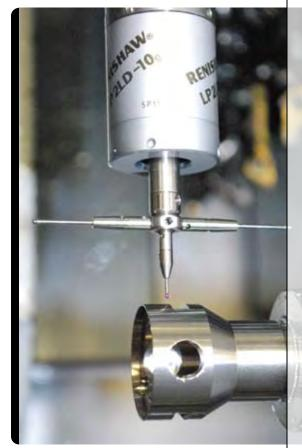
This probe installs on the platen of a Swiss-type lathe so both X- and Y-axis movement is possible. That motion combined with the probe's three styli allows access to features of parts located on both the main and secondary spindles.
