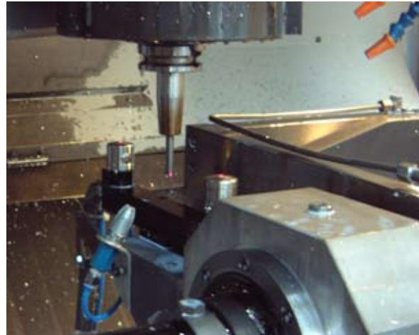
The red spot is the answer: measuring the tool length in automatic cycles ensures automatic compensation for thermal growth and therefore much greater process stability.
