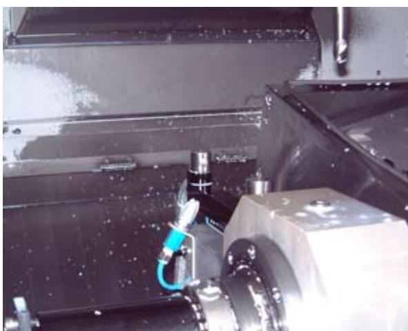
Compact and robust: the NC4 laser measuring system needs little space, has optimum chip and coolant protection, and measures with precision independent of environmental effects.
