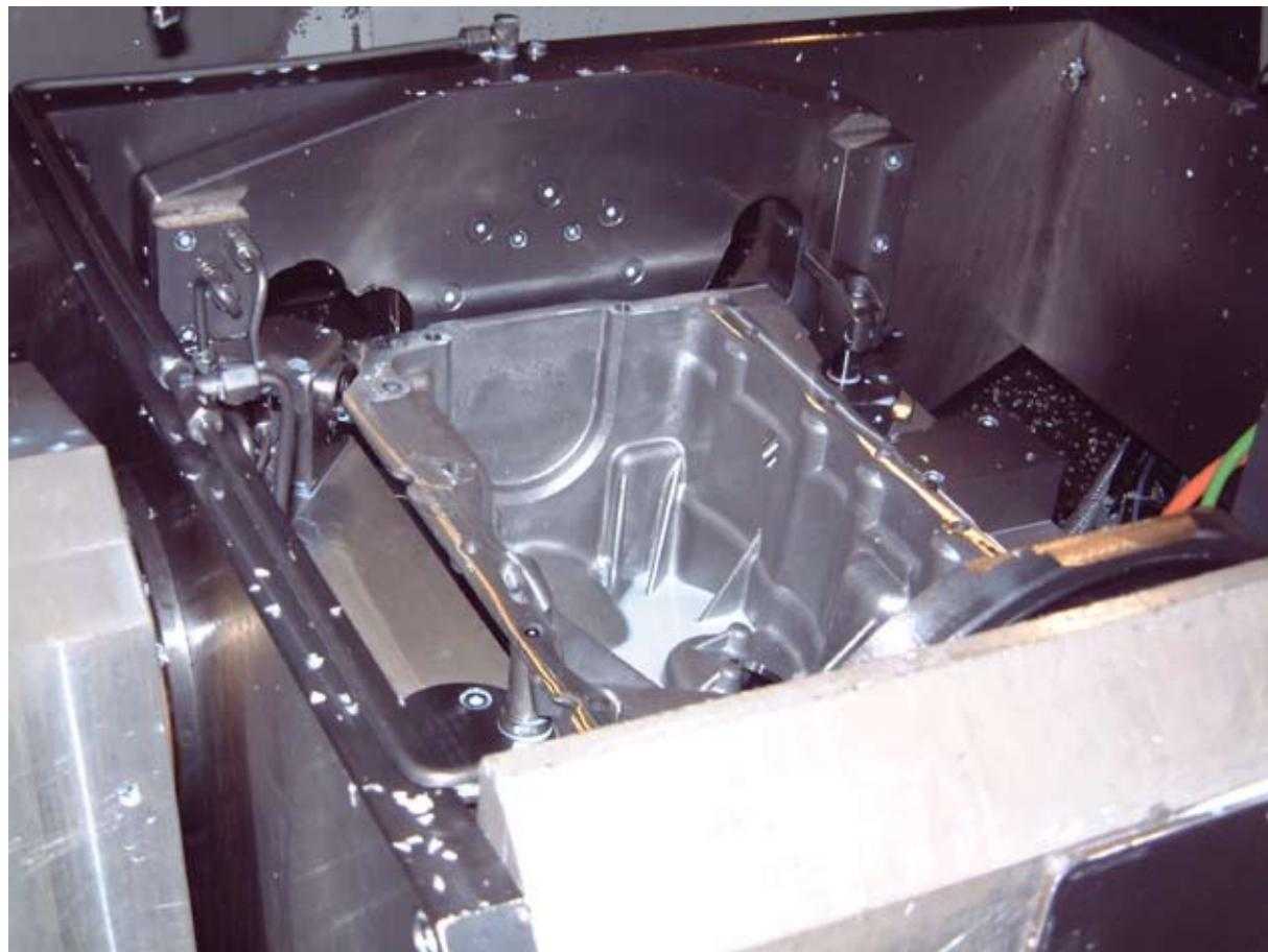
The automotive sector demands the utmost quality and process stability for the large-scale production of oil pans for internal combustion engines.
