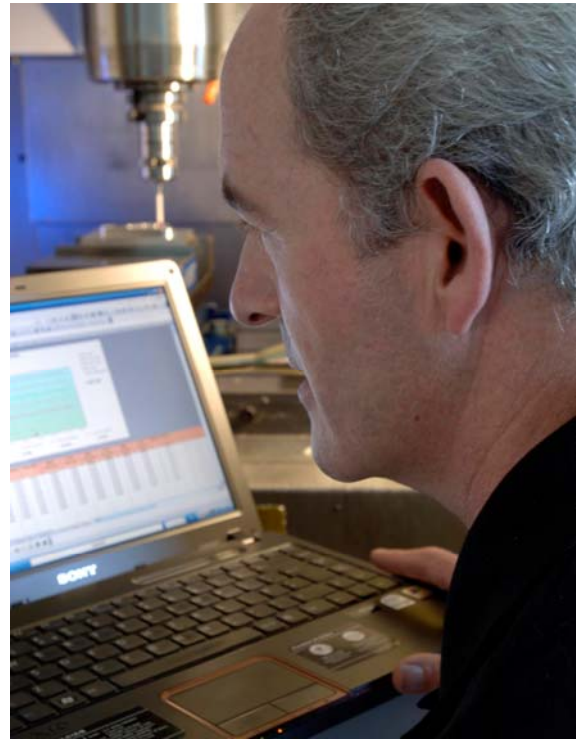
Ray Blowick uses the latest software to program the whole machining process, including the probing moves
