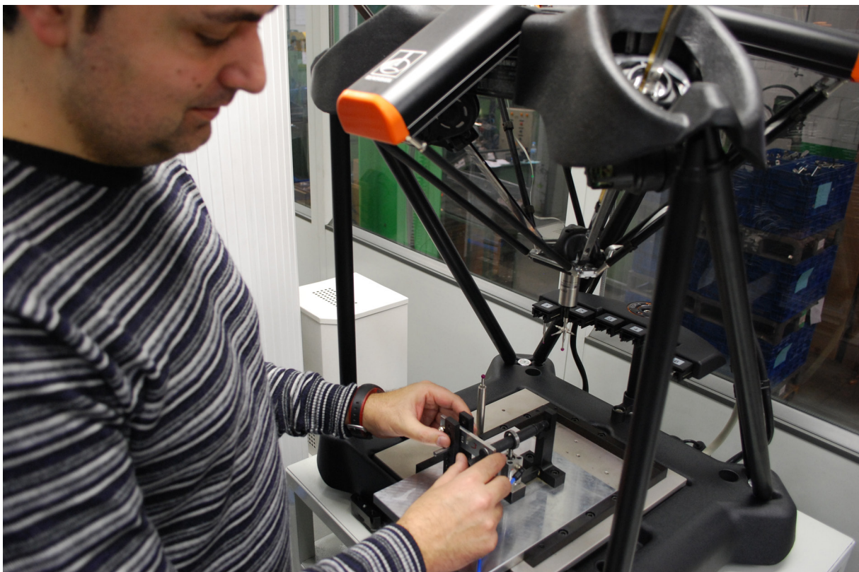
An Eponsa engineer loads a wiper mechanism part onto Equator ready for gauging.
