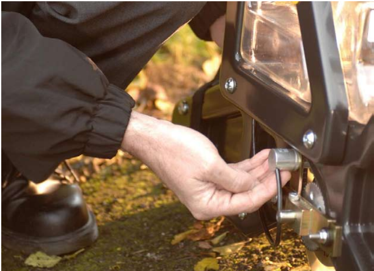
The Sperry Walking Stick uses Renishaw RE22 magnetic rotary encoders to process signals and in combination with GPS, record auditable data about crack location
