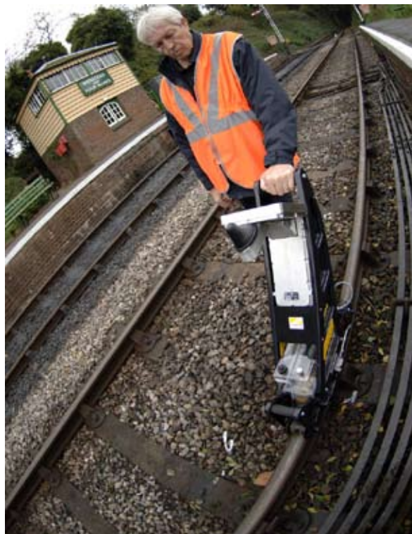
The Sperry 'Walking Stick' is a pedestrian inspection tool which the operator pushes along the railway track
