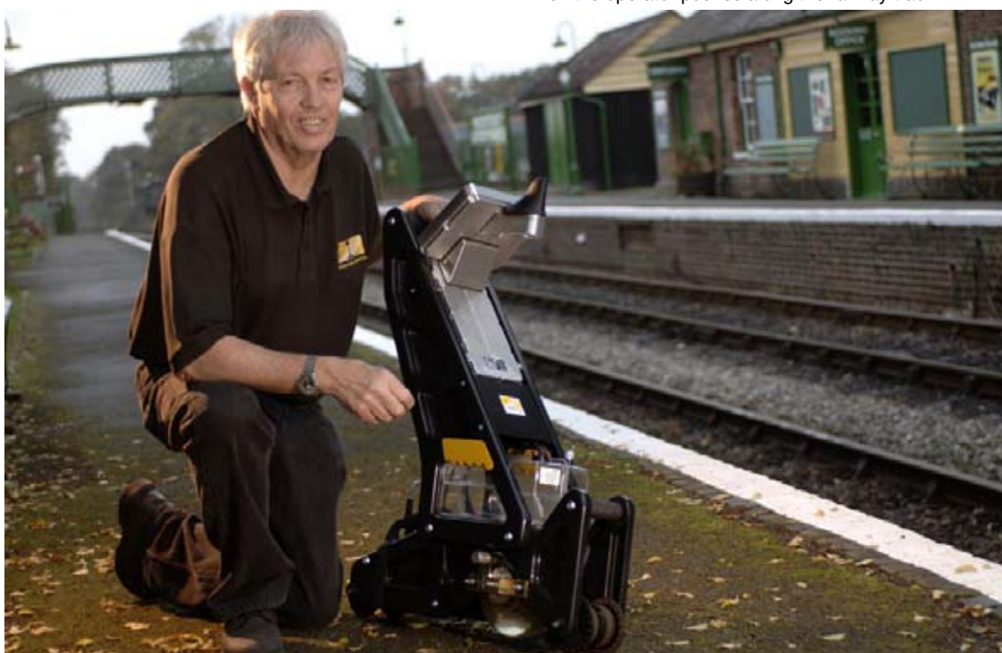
George Dodd, Field Service Manager for Sperry International, with the company's Walking Stick. It uses nine transducers to project sound into the rail to detect anomalies caused by cracks
