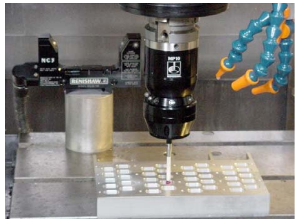
MP10 spindle probe setting a pharmaceutical part, the NC3 non-contact tool setter in the background
