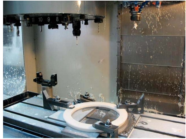
Large plastic part machined accurately with the help of ballbar
