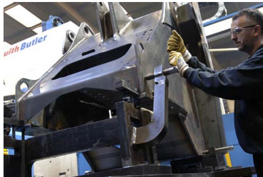
Rare variations in welding and clamping can be picked up by the Renishaw touch probe to guarantee the accuracy of finished machined surfaces
