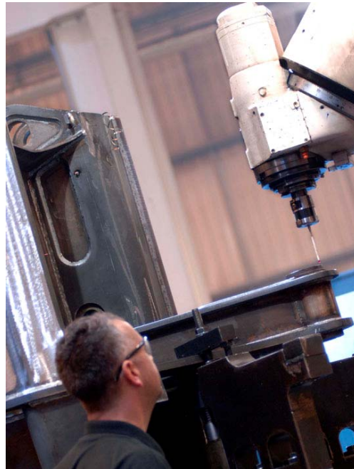
Chassis fabrications are measured before machining and programs adjusted for surfaces out of position – occasionally parts are rejected, saving hours of machining
