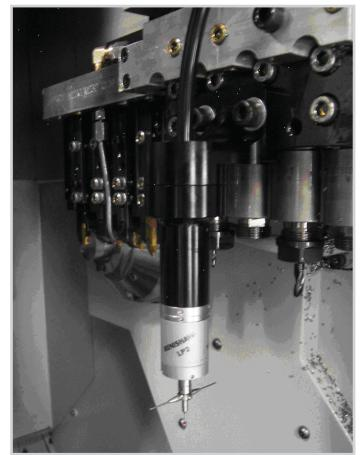
Platen-mounted probe with a 'T' stylus can access all features on complex parts.
