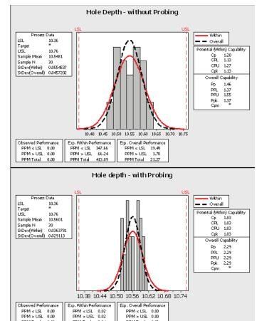
Significant improvements in process capability resulting from automated in-process control.
