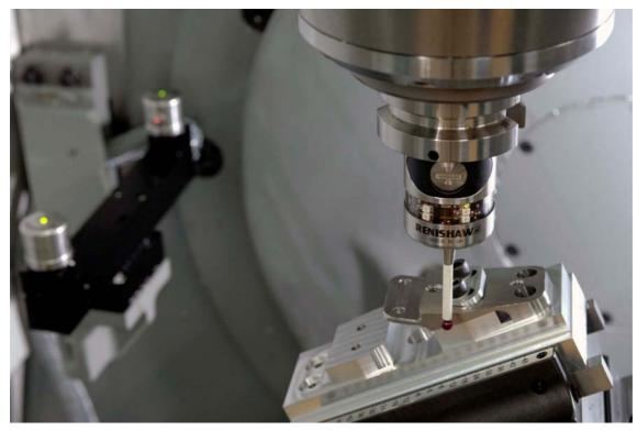
Renishaw NC4 non-contact tool setter for setting tools and monitoring for tool breakage, and OMP40 spindle probe for setting the part datum
