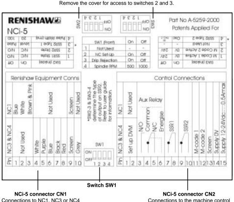
Switch settings Remove the cover for access to switches 2 and 3. Renishaw plc
