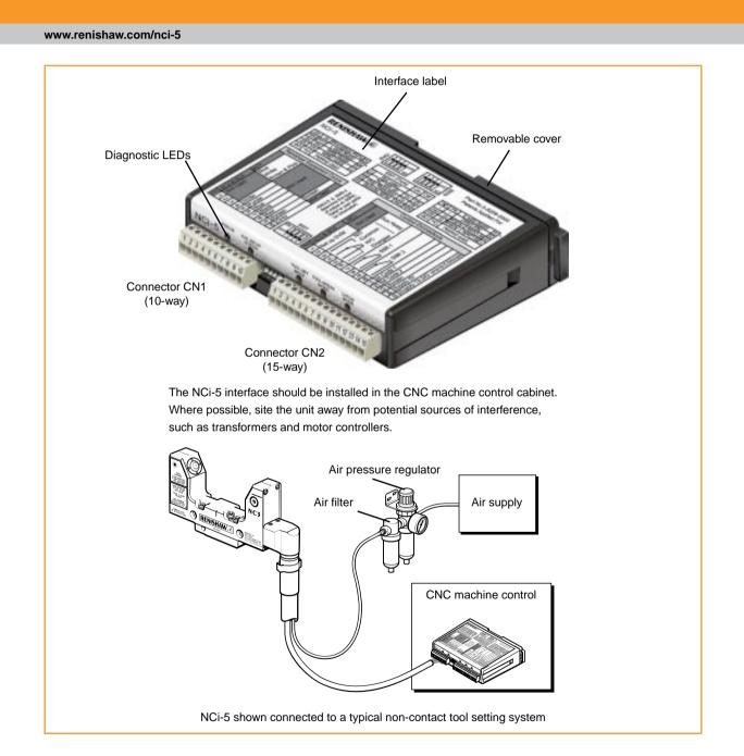
The NCi-5 interface is used with Renishaw's NC1, NC3 or NC4 non-contact tool setting systems. It processes signals from the non-contact unit and converts them into voltage-free solid state relay (SSR) outputs, for transmission to the CNC machine control. The NCi-5 features a drip rejection mode allowing it to filter out random drops of coolant without triggering the system.
