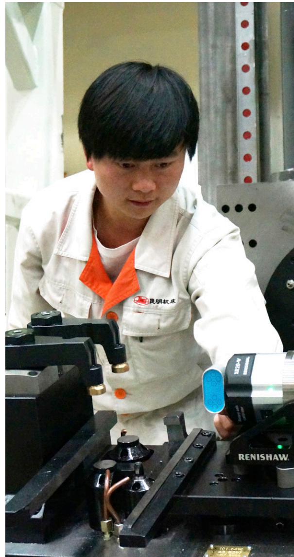
Rotary axis calibration on a machine tool using XR20-W
