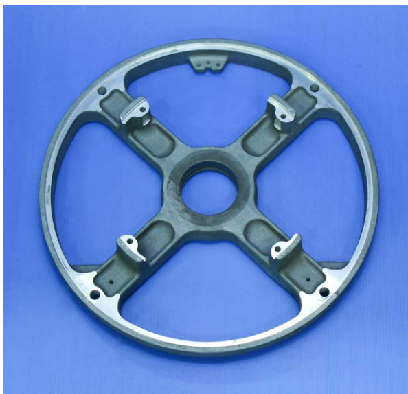
A machined endbell as used in genset engines
