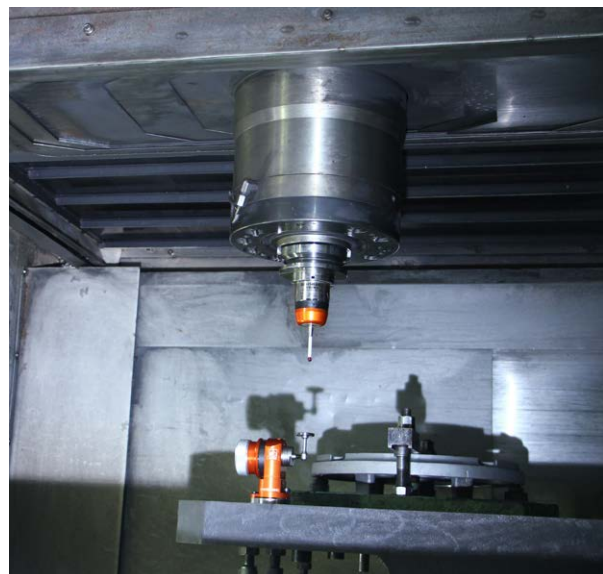
The Radio Tool Setter and Radio Part Setter on-machine at Victory Precisions Pvt. Ltd.
