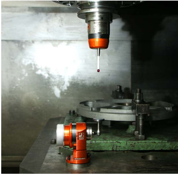
The Primo system locating positions on an endbell component
