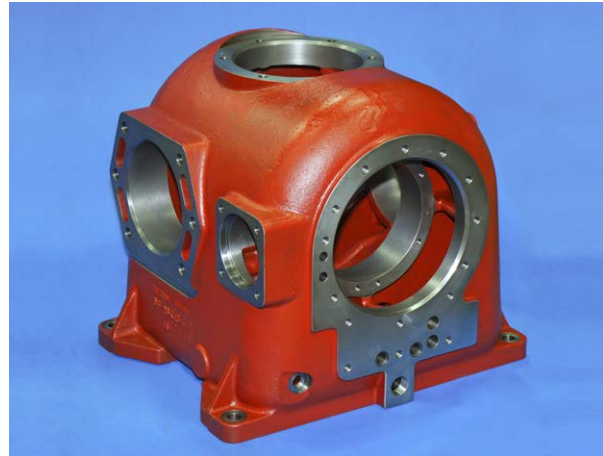
Concentricity is critical during machining
