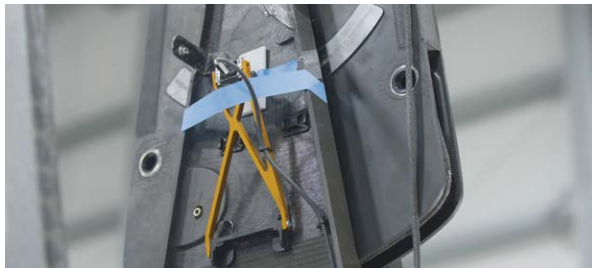
The encoders installed on a hammerhead (flap control plate)
