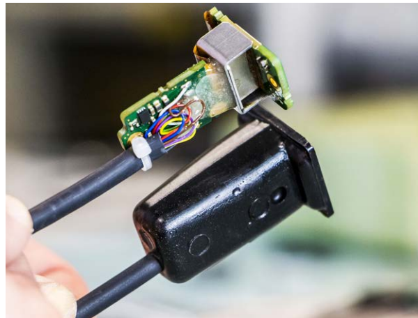
The RLS LinACE™ repackaged into a waterproof enclosure
