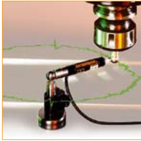
QC10 ballbar – fast machine tool performance testing
