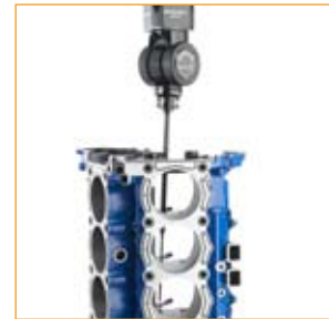
REVO™ – servo scanning head probing system
