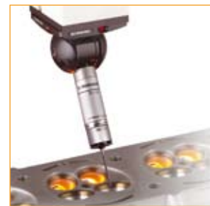
SP25M scanning probe – rapid and continuous data capture
