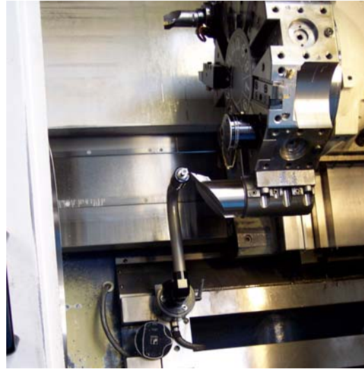
Setting tool cutting tips with a highly repeatable removable Renishaw arm
