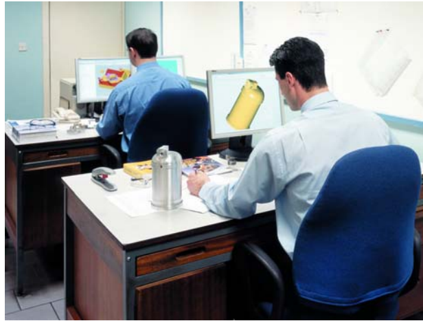
Parts are taken from original CAD drawing directly to production, with automatic generation of the machining program followed by immediate virtual 'prove-out' of the entire machining and probing cycle
