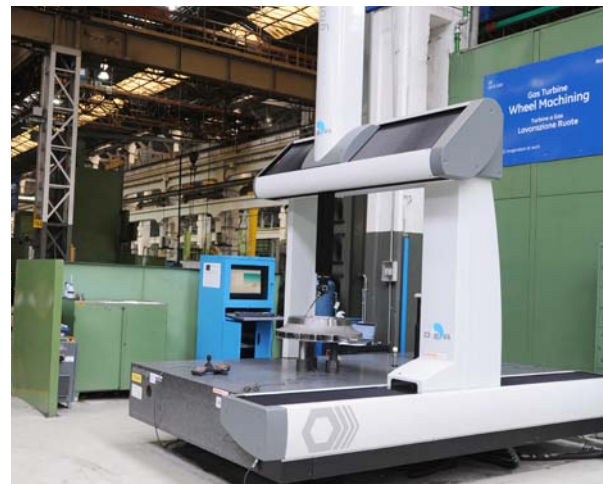
The DEA Global CMM, now capable of far higher data collection rates and form analysis
