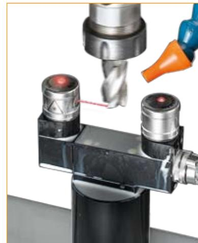
NC4 compact checking a tool for breakage
