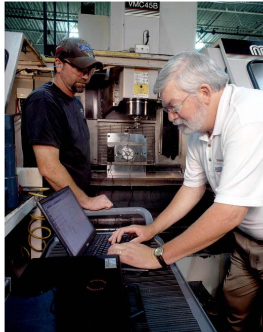
Analysing the results of the QC10 ballbar test
