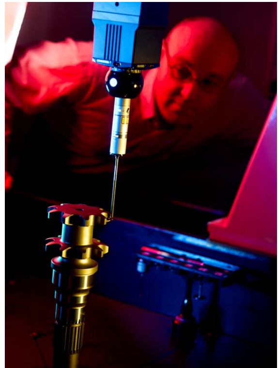
Nigel Peace, Process Control Co-ordinator, programs the inspection of a component using the Renishaw SP25 scanning probe
