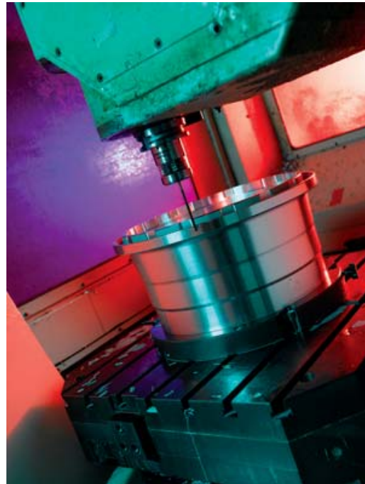
Spindle-mounted touch probe setting the machine coordinate system relative to existing machined features, ensuring machining starts in the right place every time.
