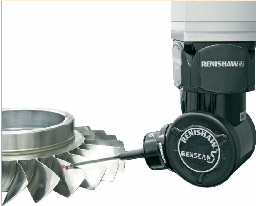
REVO™ 5-axis scanning head, with a fan blisk
