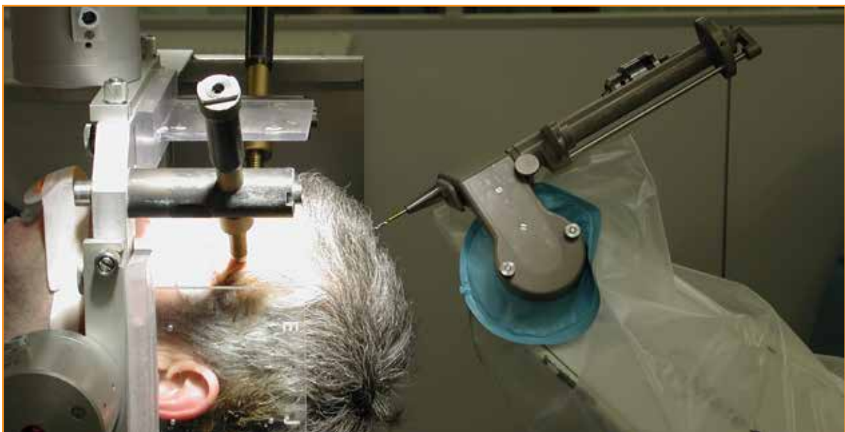
neuromate * robot with drill attachment and frame, used for reference and to rigidly support the skull
