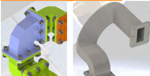
Removal of joints
