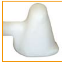
Once machining is complete, the coping is left attached to the material by means of a connector or 'spigot' (figure 3).
