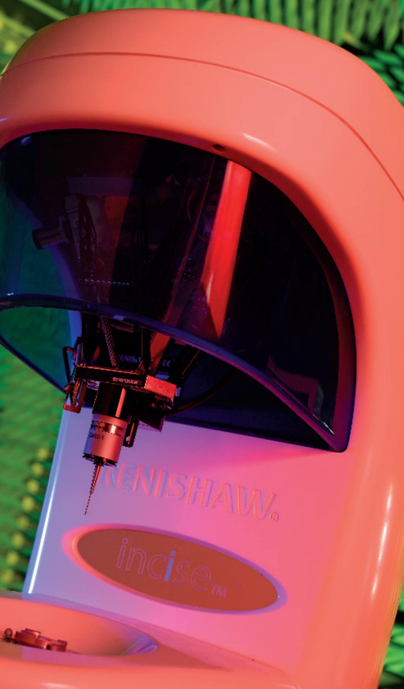
An incise™ dental scanner undergoing electromagnetic compatibility (EMC) testing in a recently installed 35 m² screened room.
