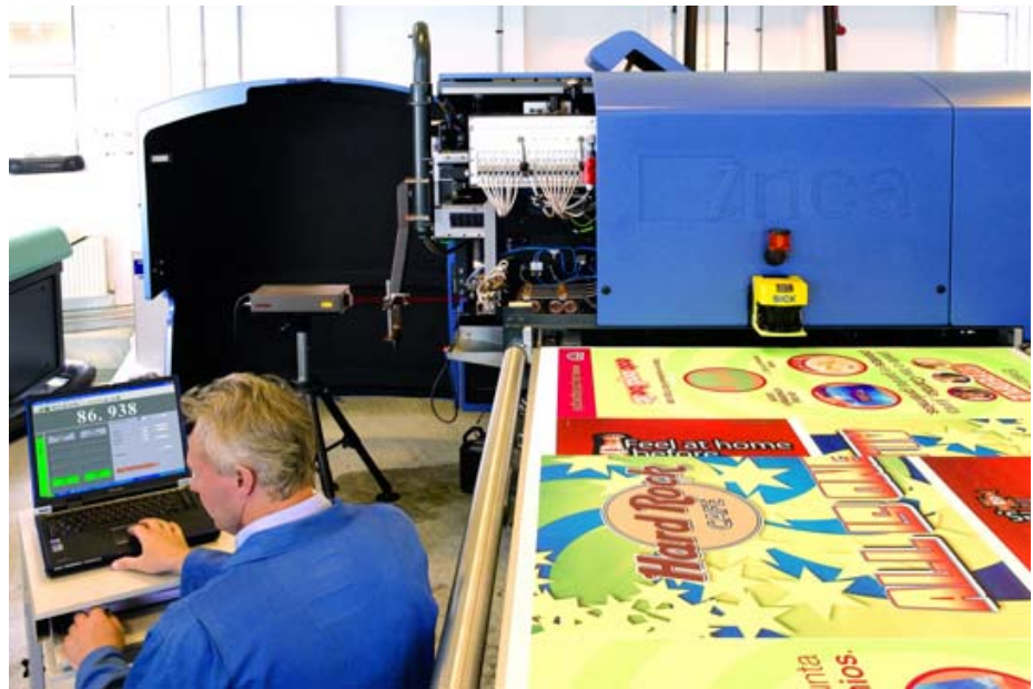
Inca flatbed printer undergoing calibration of the positional accuracy of the printing head, using the Renishaw ML10 laser measurement system.
