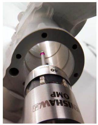
The Univer 6 machines the complete axle to a tolerance of 3 microns, drilling and rearing the mounting holes for the chassis and the bore hole for the king pin, together with a host of other operations.
