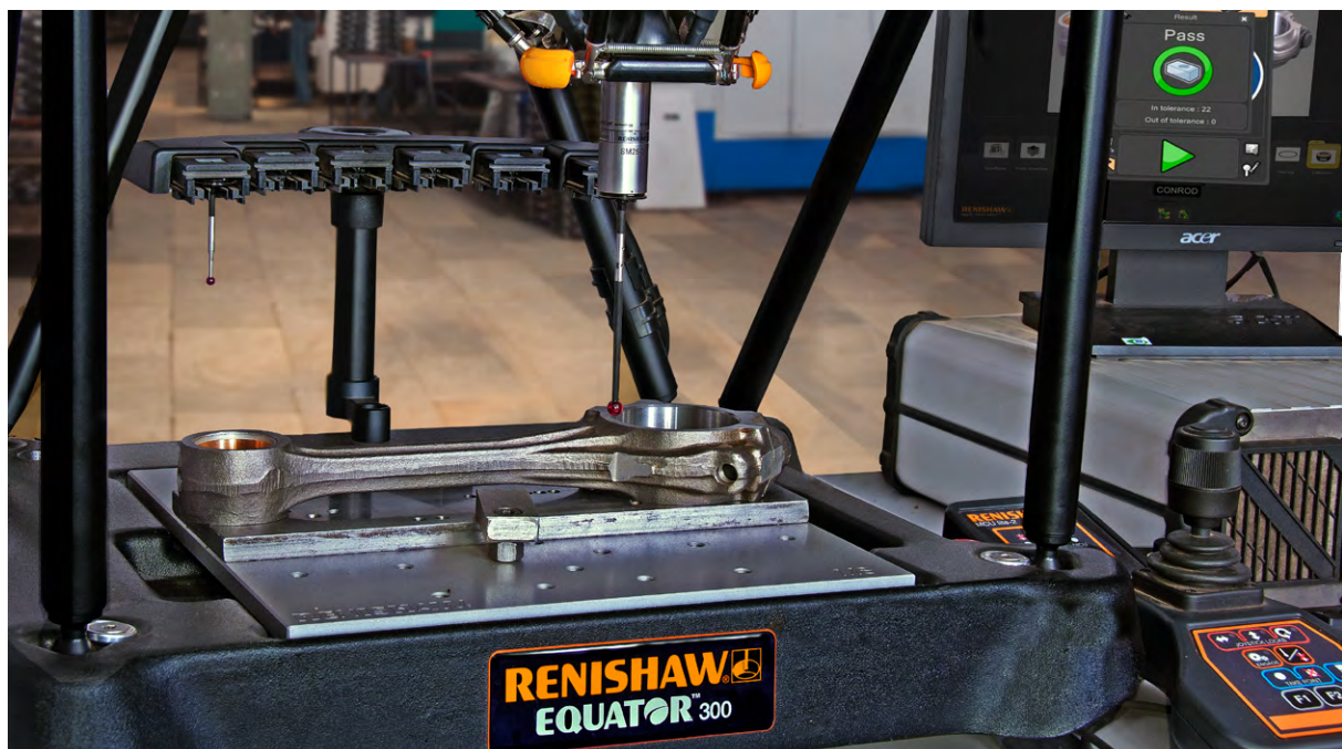
Kishan con-rod on fixture plate on Equator 300
