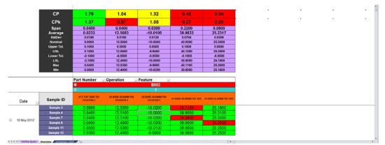
The **Overview** tab shows actual measured data in colour coded data cells indicating adherence to tolerance. (This is the same information as displayed by the **Overview** tab in Renishaw CNC Reporter.)
