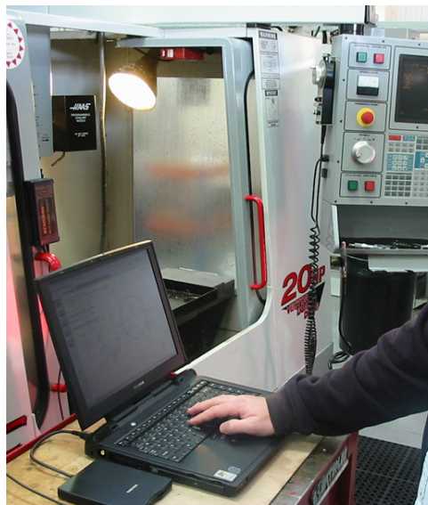
The QC10 ballbar test is controlled with software on a PC, the data gathered will then be analysed with Ballbar diagnostic software off-line
