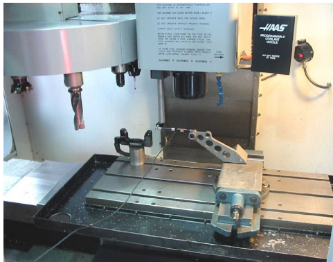
QC10 ballbar testing positioning performance on a HAAS VMC
