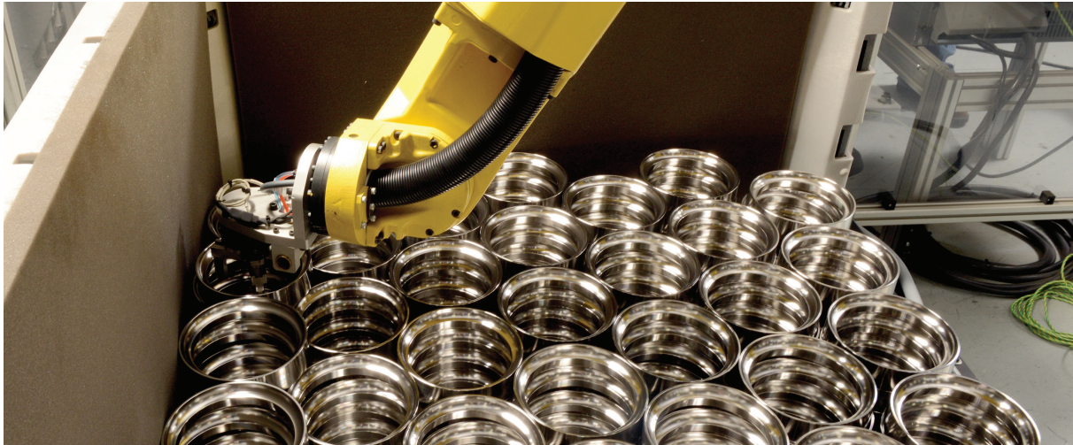
An automated FANUC robot boxes and palletises parts
