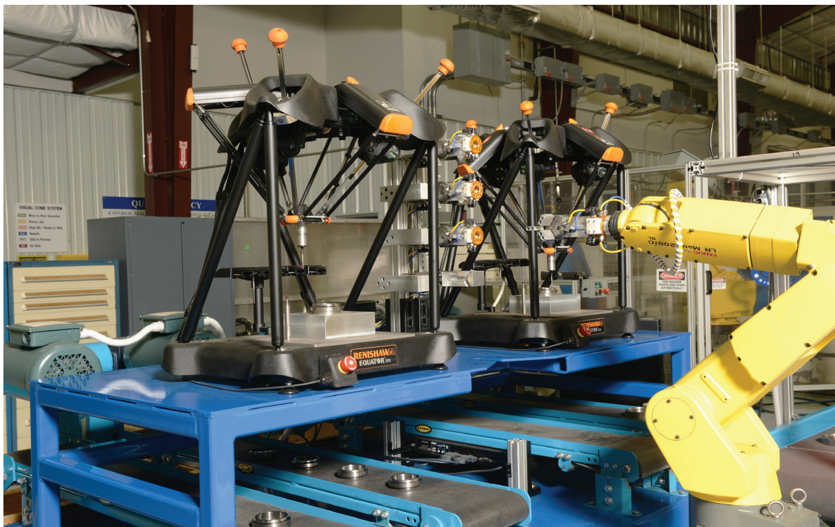
In development - Conroe's new dual Equator automated cell
