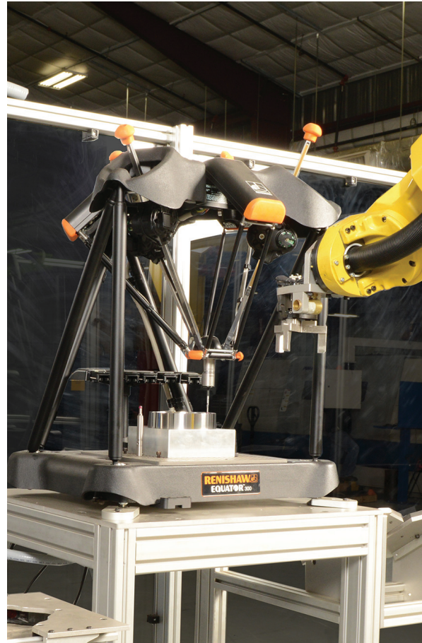
A FANUC robot loads the Equator in the automated cell
