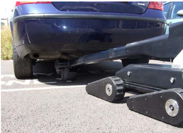
The Guardian is versatile enough to extend 2.6m high or inspect under cars.
