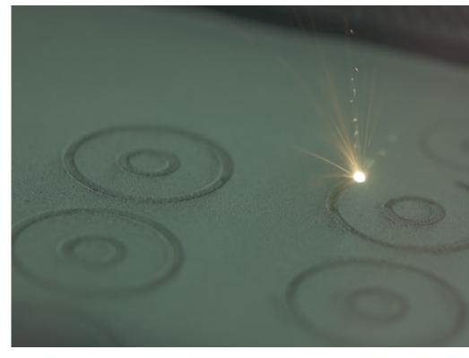
The collaboration between Domin and Renishaw has led to significant improvements in operational efficiency. One of the important outcomes has been the dramatic increase in production throughput, around 120 metal AM manifolds are now being printed every day.
