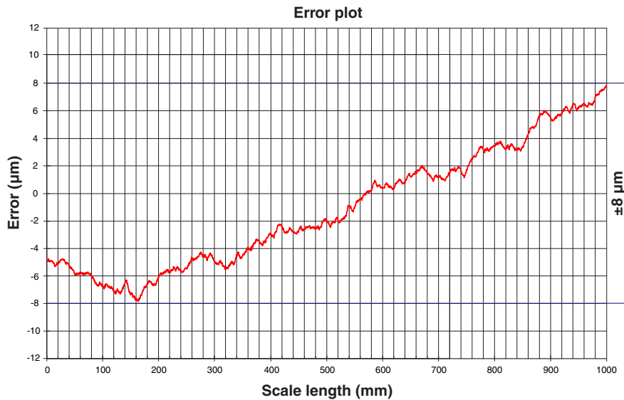
Example accuracy test result of 1000 mm length of RTLA50 scale
