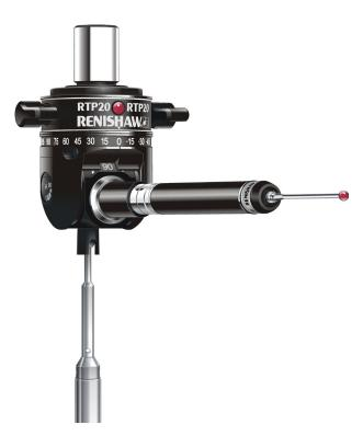
RTP20 integral TP20 probe mount optimises the working volume of the CMM and provides compatibility with all existing TP20 modules. Although modules can be changed manually, the RTP20 can be used with the MCR20 module change rack, allowing fully automated module changing.
