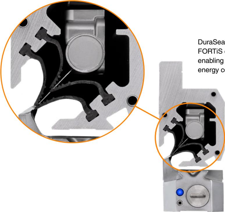
DuraSeal™ lip seals have been specially developed for FORTiS encoders and provide superior sealing properties, enabling operation with lower air consumption, reducing energy costs and carbon footprint.
