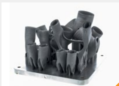
Build plate showing a set of titanium lugs for a bespoke mountain bike.
