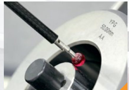
Precision styli ensure accurate acquisition of measurement data.
