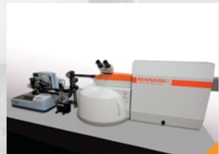
inVia Raman microscope integrated with a Bruker atomic force microscope.
