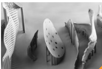
Titanium craniomaxillofacial implants produced using a Renishaw metal additive manufacturing system.
