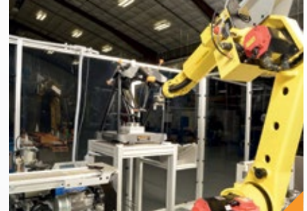
Equator™ gauge integrated within a robot-loaded manufacturing cell.
