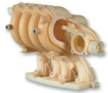
Prototype manifold produced by a vacuum casting machine.
