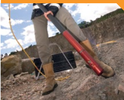
Deploying a C-ALS system for measuring underground voids.
