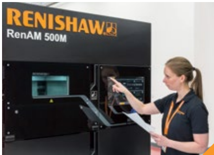
Additive manufacturing machines build components up layer by layer.
