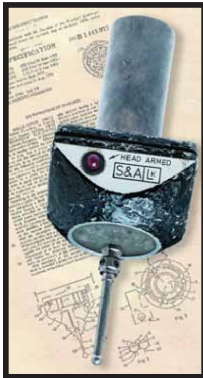
First 3-D touch-trigger probe and patent by Sir David McMurtry.
