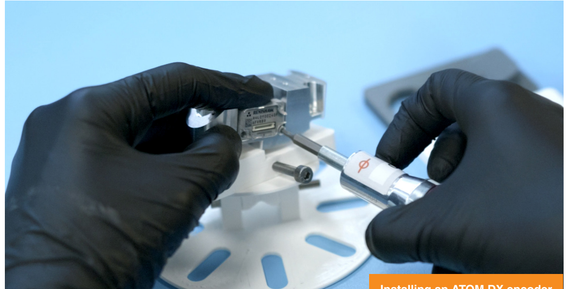
Installing an ATOM DX encoder
