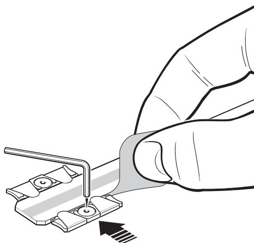
4. Place the datum clamps against the scale and secure them using the special M3 low-profile screws supplied.
