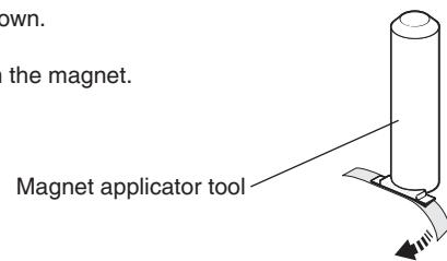
3. Place the magnet on the scale ensuring it does not impede the incremental track as shown below.
