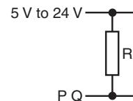
**NOTE:** Select R so that maximum current does not exceed 20 mA. Alternatively, use a suitable relay or opto-isolator.
