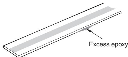
7. Allow 24 hours for the epoxy to cure fully then clean the scale using the Renishaw scale wipes or a clean, dry, lint-free cloth.
