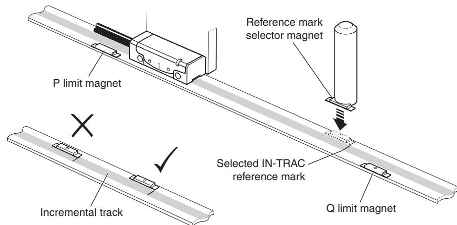
**NOTE:** The reference mark selector and limit actuator locations are correct for the readhead orientation shown.
