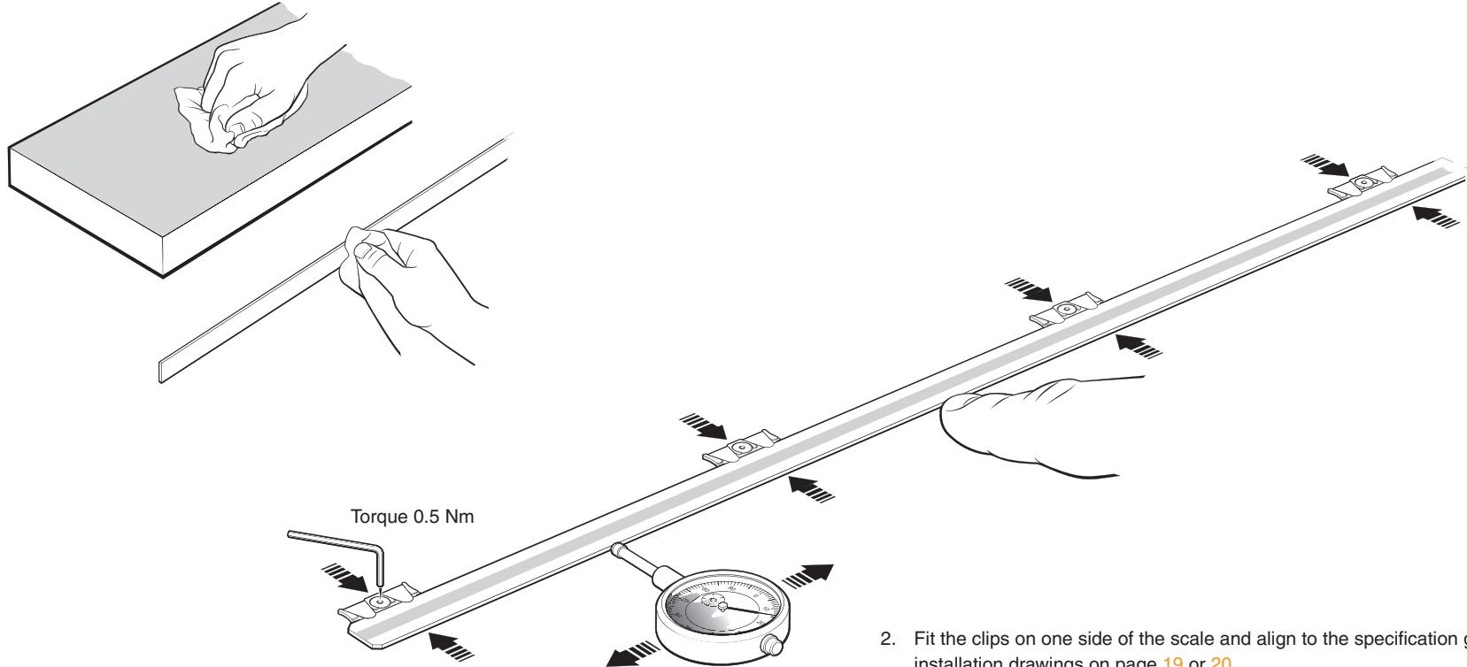
2. Fit the clips on one side of the scale and align to the specification given in the relevant installation drawings on page 19 or 20.
