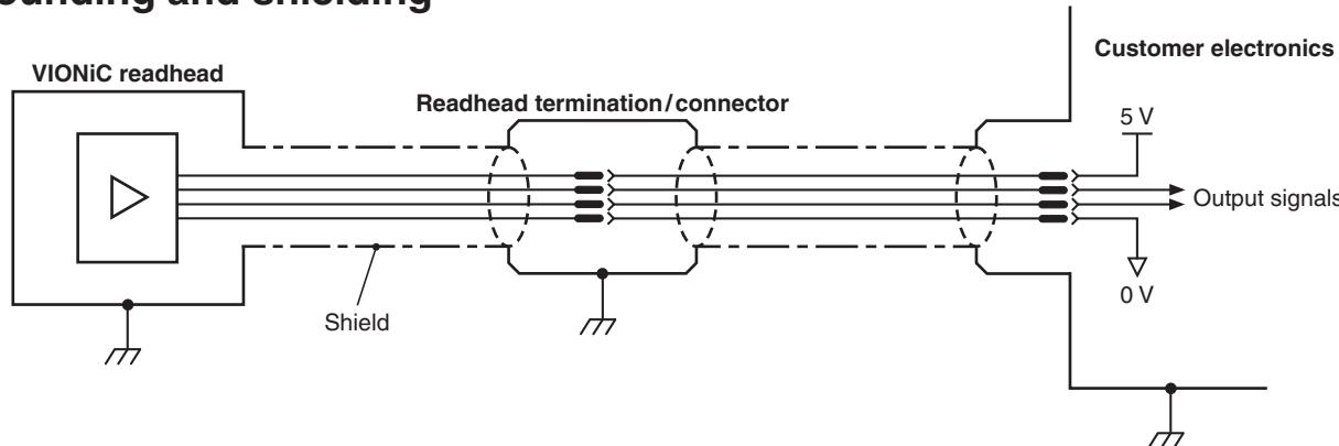
**IMPORTANT:** Connect the shield to the machine earth (Field Ground). For JST variants connect the ferrule to the machine earth.
