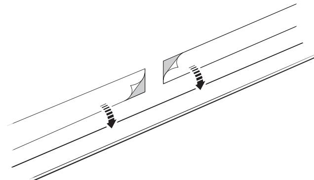
4. Thoroughly mix and apply the epoxy to the back of the scale and then remove the remaining backing liner.
