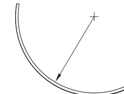
**NOTE:** During storage make sure the self-adhesive tape is on the outside of the bend.
