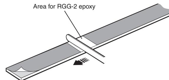
5. Locate the scale against dowels or a ledge and rotate it down onto the substrate. Press down firmly.
