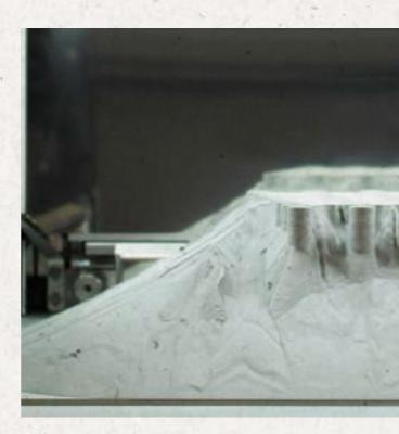
Renishaw also designed support structures to enable easy powder removal.
