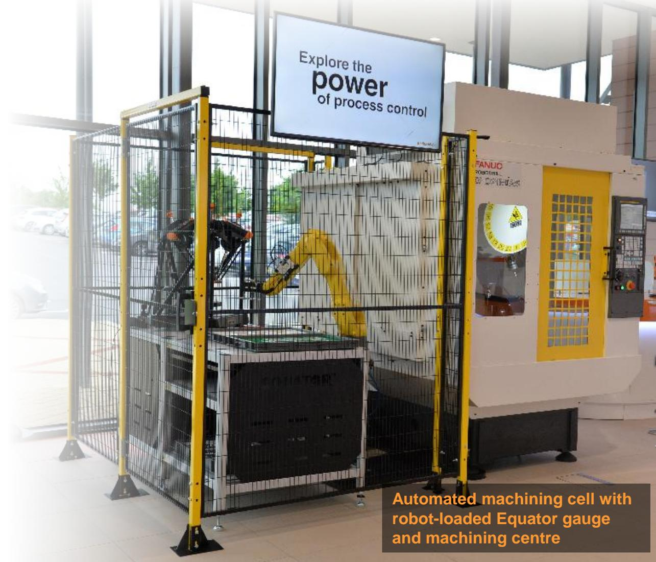
Automated machining cell with robot-loaded Equator gauge and machining centre
