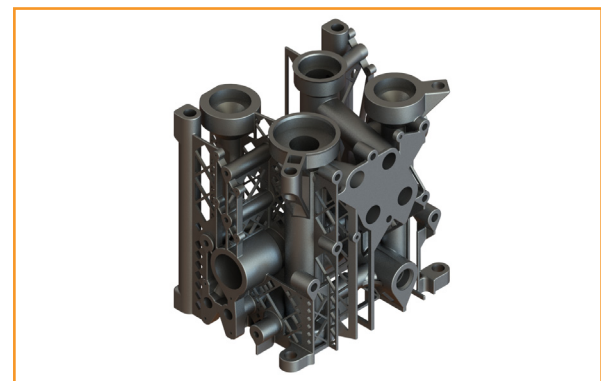
First iteration geometry. Flow paths have been extracted, optimised and wall thicknesses applied. Support structures act to hold the flow paths in place and connect fixture points
