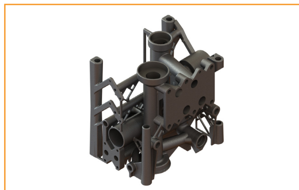
Second iteration geometry. The block extraction passages have been removed and the support structures reworked for increased stiffness and rigidity
