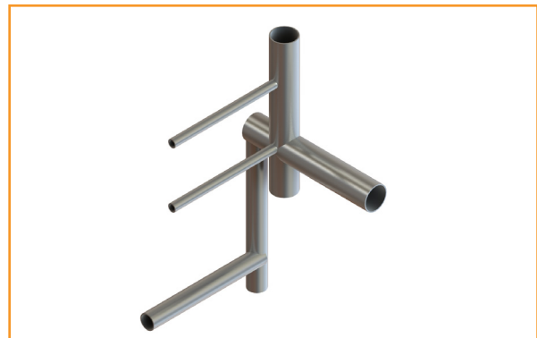
Extracted flow path section highlighting abrupt junctions
