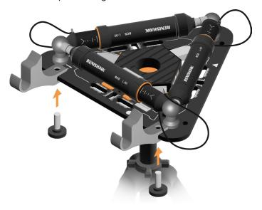
3. Place the calibrator into the brackets.
