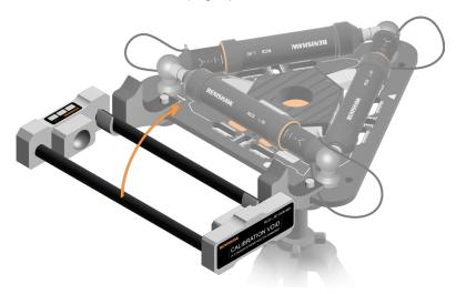
5. Tilt the calibrator towards the baseplate until it is stopped by the brackets. This prevents the calibrator from rolling backwards.
