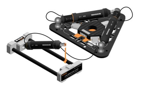
Extend the ballbar so that the opposite end reaches the opposite ball surface of the calibrator. Ensure the RCS L-90 ballbar is magnetically attached to the calibrator.
