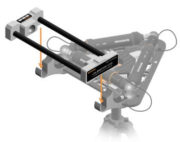
4. Rotate the calibrator to the upright position.
