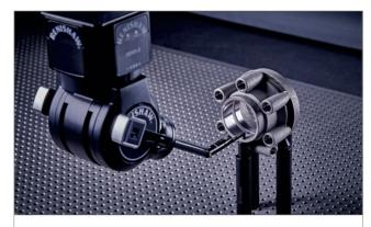
Our products enable customers to maximise the potential of their capital equipment; the REVO-2 measuring system for CMMs allows a range of inspection applications on a single machine, including dimensional and surface finish measurement.
