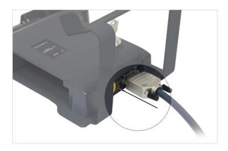
4. Press and hold the recessed switch at the back of the MCU W cradle until the blue pairing status LED starts to flash rapidly, this should be about five times a second.
