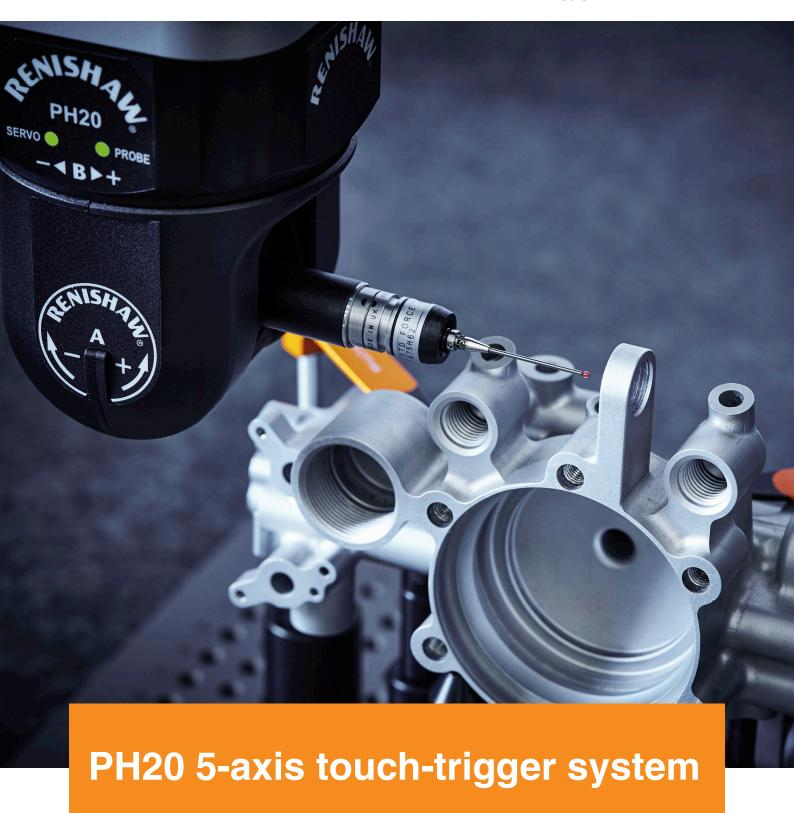
Fast, accurate 5-axis technology for touch-trigger applications on all sizes of CMM
