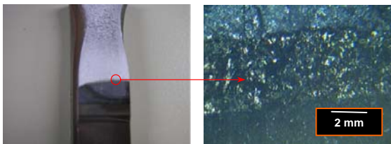
Figure 11 The image left shows the part that had been withdrawn from service and the interface between the unaffected and oxidised regions. The low power optical micrograph on the right shows a higher magnification image of the interface
